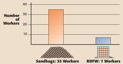
RDFW vs. Sandbag Comparison: 100-foot wall, 4 feet high
